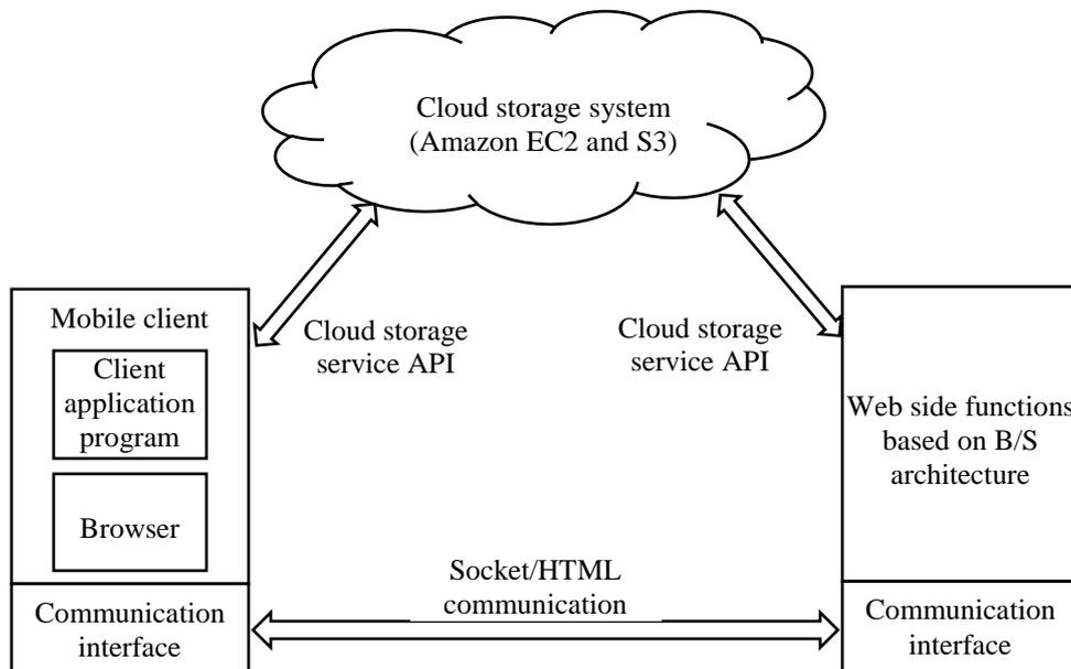
Figure 2: The system architecture of the network teaching platform based on mobile cloud computing.
